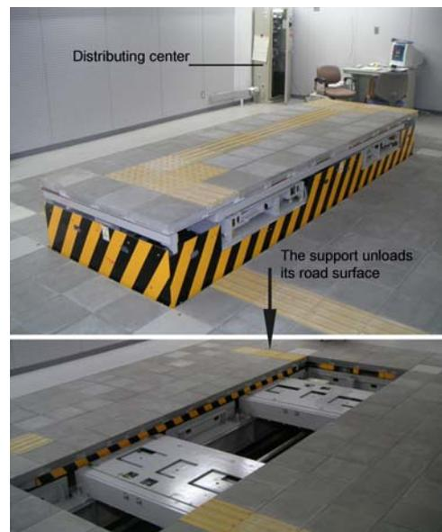
Fig. 1: Road surface and its support.
