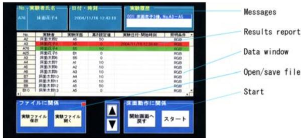
Fig. 5: Automatic model controllers (in Japanese).
